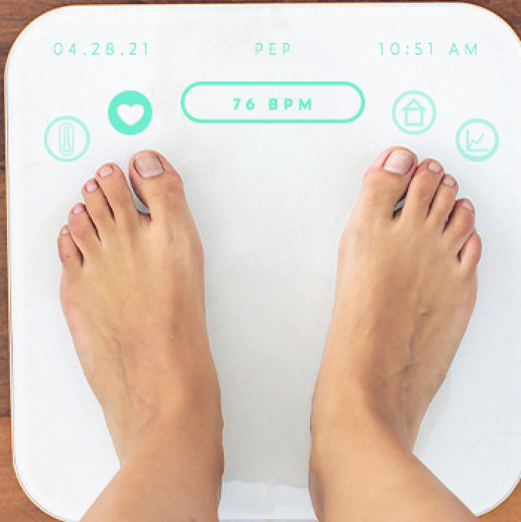
The scale also shows the basic reading for the designated page for easy viewing. Seen on top of the scale display is the date and time as well for additional info.
